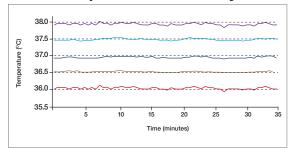
The incubation chamber's temperature uniformly cools or heats samples to within  $\leq \pm 1.0^{\circ}$ C.
