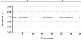
With a <±0.3°C (high temp.) and <±0.5°C (low temp.) temperature stability BEING ensures experiment stability.
