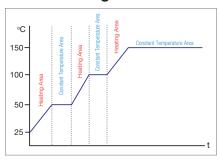
In program control mode, the controller allows the operator to set up step cooling and heating control.
