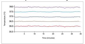
The incubation chamber's temperature uniformity enables all samples to be heated evenly.
