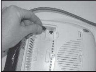
3. Connect the battery pack cable to the unit's battery connector in the bottom of the battery recess.
