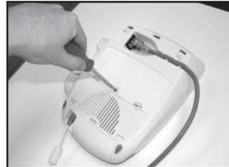
5. Replace the battery access door and re-tighten the screw using the screwdriver.
