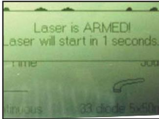
5. Press the START button. A message displays to alert you to the fact that the laser is armed. The unit will beep two times to count down the number of seconds left until the applicator is ready, and an orange light will blink two times on the back of the applicator. Press the Pause/Resume button to begin the treatment.
