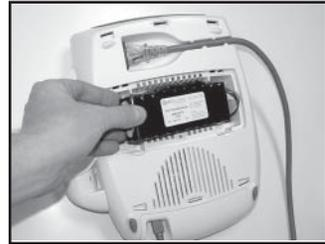
4. Put the battery pack into the unit, making sure to orient it as shown.
