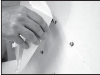
7. Line up the screw heads with the holes on the repositional base, and slide the unit down slightly until the screw heads are securely fastened to the repositional base.
