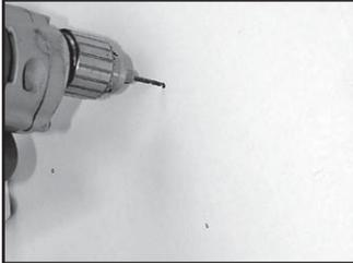
3. Using a 9/64 (3.6 mm or 0.357 cm) drill bit, drill four holes you marked in the previous step.
