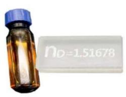
Bromonaphthalene nD = 1.51678 Refractive index standard kit is the calibration standards are for the calibration of refractometers. This refractive index standard kit is measured by means of an Abbe type refractometer or other type refractometers.
